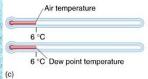
Saturation specific humidity =  $6 \frac{\text{g}}{\text{kg}}$
