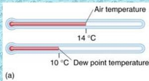
Saturation specific humidity =  $10 \frac{\text{g}}{\text{kg}}$
