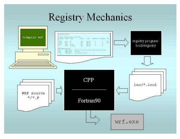
Figure 8.1. When the user compiles WRF, the Registry Program reads Registry/Registry, producing autogenerated sections of code that are stored in files in the **inc** directory. These are included into WRF using the CPP preprocessor and the Fortran compiler.
