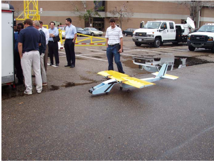
Unmanned aerial vehicle developed at LSU for taking high-resolution pre- and post-storm imagery.
