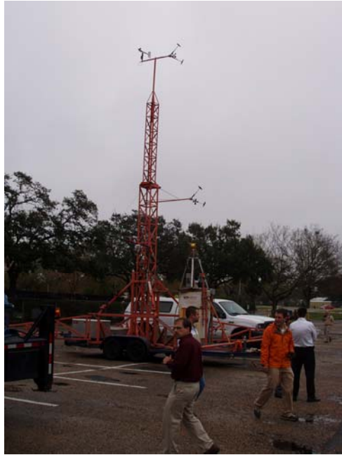
One of the Florida Coastal Monitoring Program's portable instrument towers
