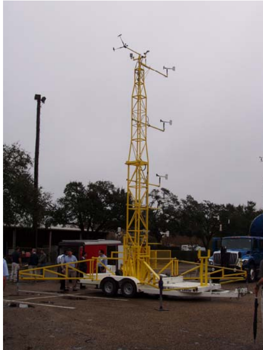
Louisiana State University's (LSU) STORM 1 mobile instrument tower. This is the first tower built by LSU to study landfalling tropical cyclones.
