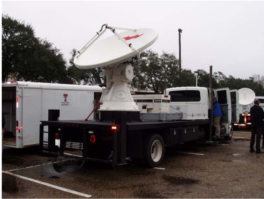
The NOAA XP Mobile X-Band Dual –Pol radar on display. Radar is operated in conjunction with the National Severe Storms Laboratory and the University of Oklahoma
