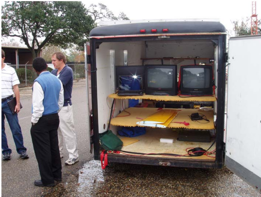
Control and support trailer for the LSU UAV, providing real-time imagery during each flight.
