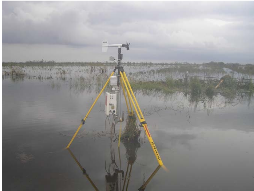
Photo of probe 0105A 6 miles east of Winnie, TX along SR 73. It appeared that the probe was experienced approximately 3.5 ft of storm surge flooding. At the time of retrieval approximately 1.5 ft of water was still over the feet of the probe. The probe functioned properly and collected a complete data record through the peak of Hurricane Ike. Photograph was taken during the afternoon on September 15, 2008 by Tanya Brown.
